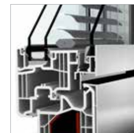
FLUSH DESIGN With this innovative composite window in modern square-edged design, integration into the facade is possible on three sides. Inside with square-edged glass bead
